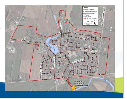
Finally, let's look at the wastewater collection system. This is the network of pipes that take the community's sewage to the wastewater treatment plant. What you see here is our network of wastewater pipes that run under the roads of the Village.
